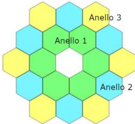
**Fig. 6.** The ring diagram for the primary mirror. The mirrors of the first ring are shown in green, second ring in light blue and third ring in yellow.
