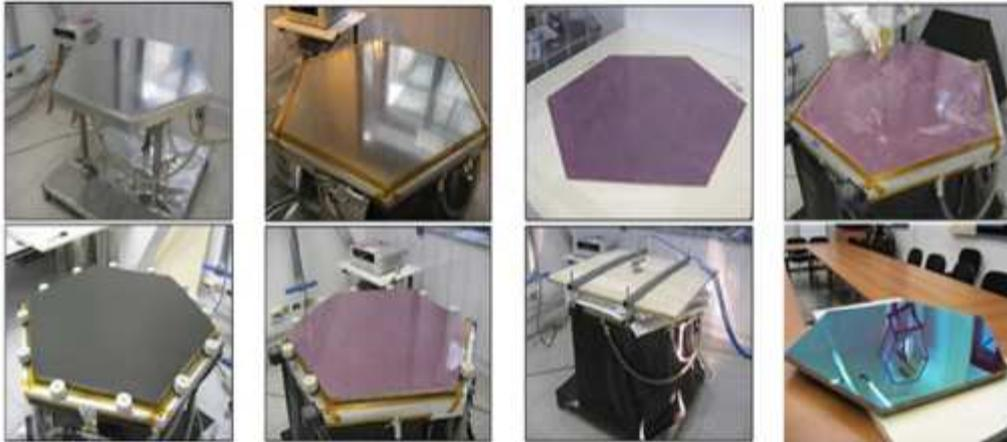
**Fig. 10.** The production process of the panels of the primary mirror.
