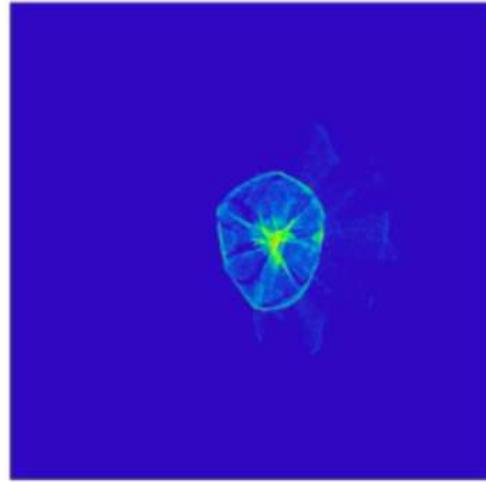
**Fig. 7.** Image of a point-like source obtained when all the primary mirror panels are aligned.
