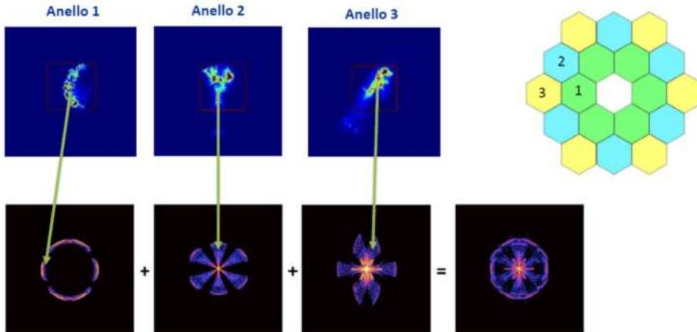
**Fig. 8.** Images of a point-like source produced by the mirrors belonging to the different rings. Top row, from left to right the image produced by a panel of ring 1, 2, 3 respectively. Bottom row, the combined images produced by the mirrors in the various rings and the final image. The images on the top row are real images while those on the bottom are simulations.
