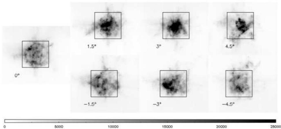
**Fig. 11.** Images (PSF) of a point-like source (Polaris star) obtained moving a CCD camera along the field of view of the ASTRI-Horn telescope.
