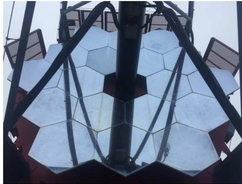
**Fig. 5.** The segmented primary mirror of the ASTRI-Horn prototype telescope.
