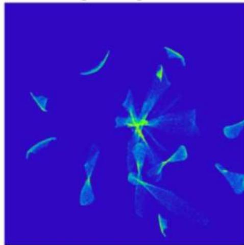
**Fig. 9.** Image of a point-like source obtained when the panels of the primary mirror are misaligned.
